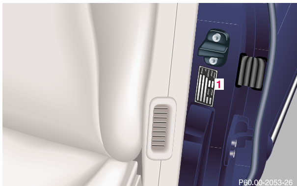
1 Certification label (below driver's door lock latch)
